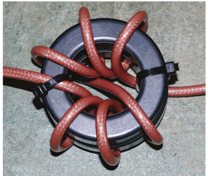
PHOTO 1: A 7-turn broadband common-mode choke.
