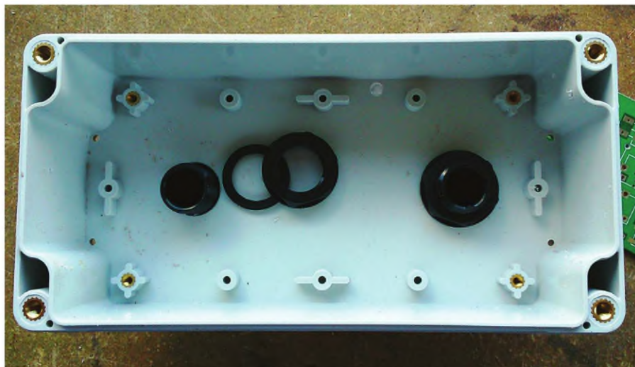
PHOTO 4: Installing the cable glands. Note the four small drainage holes drilled at the widest points of the box.
