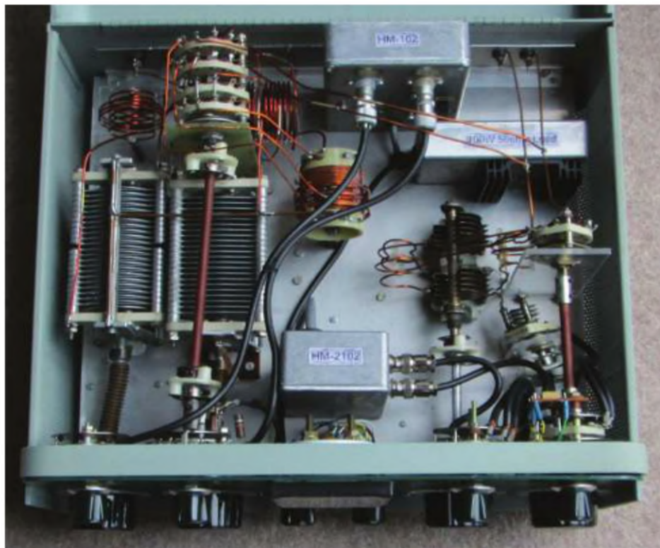
PHOTO 2: Top view of chassis layout showing the modifications to the HF tuning capacitor C2.
