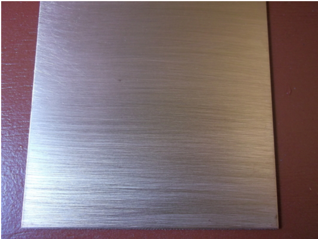
Figure 5.4: Board Cleaned with 3M Pad.
