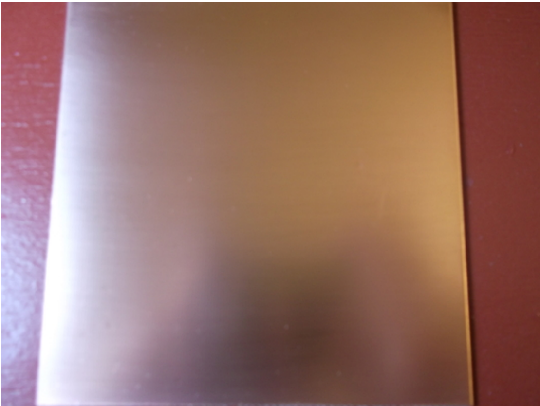
Figure 5.5: Board Cleaned with Steel Wool.
